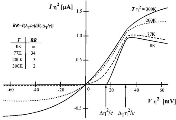
FIG. 2.  $I$ - $V$  characteristics of a WN junction for various temperatures. For the widths of the wide and narrow leads we take  $d_W/d_N(=\Delta_T/\Delta)=2$  and  $d_N=20a$ . The scaling factor is defined as  $\eta=d_N/(20a)$ . Values for the rectification ratio  $RR$  of this structure are given in the inset.
