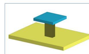
Optical Lithography + Reactive Ion Etching + KOH @70°C
