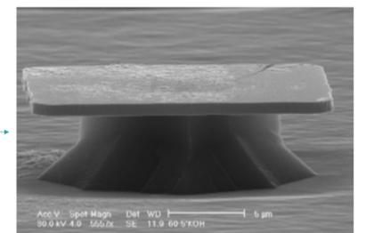
Substrate-anchored membranes are obtained!
