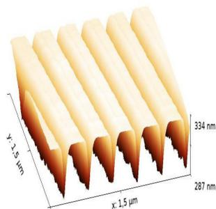
SEM and AFM images shows the obtained patterning: long ridges separated by gaps of a few tens of nanometers.
