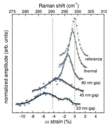
a uniaxial tensile strain of the order of 4% has been observed
